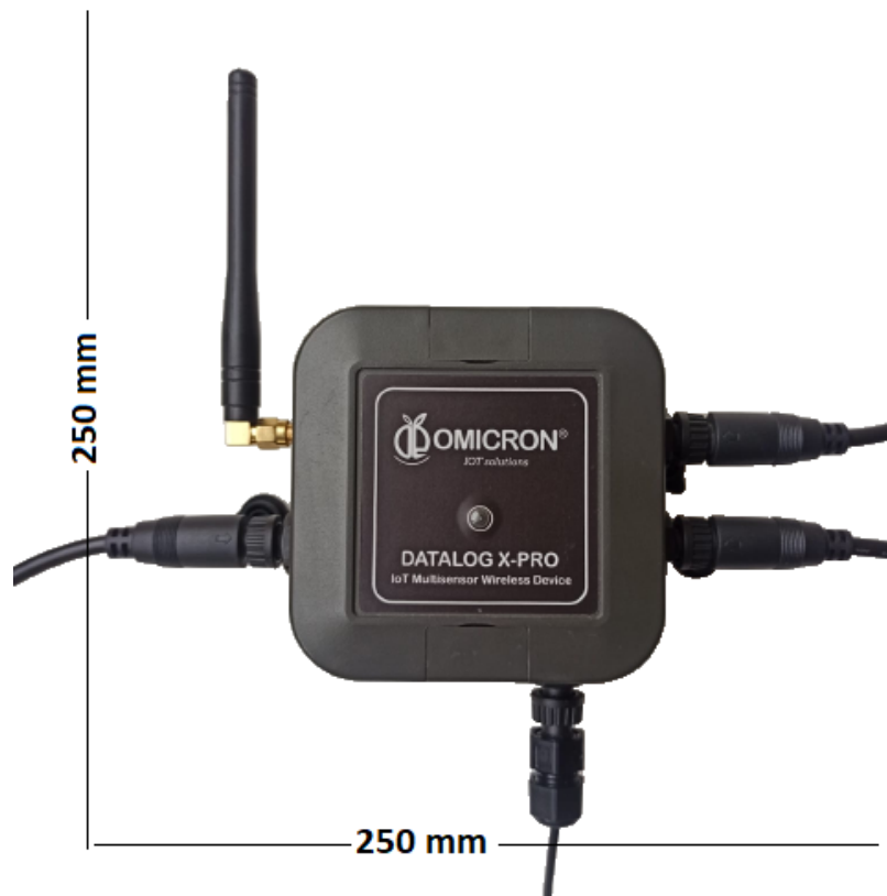
Figure 2-6 Recommended free space around the Datalog X-PRO
