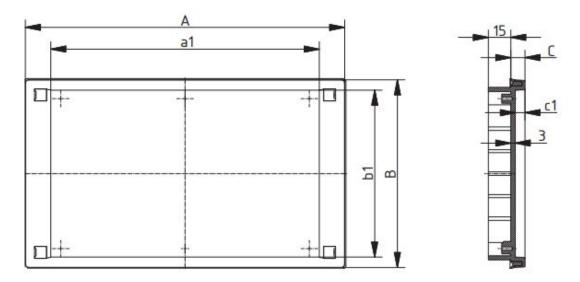
Material: ABS (IP54). A=166mm B=106mm C=9.5mm a1=131.3mm b1=92.3mm c1=6.5mm. **Total weight:** 165g.
