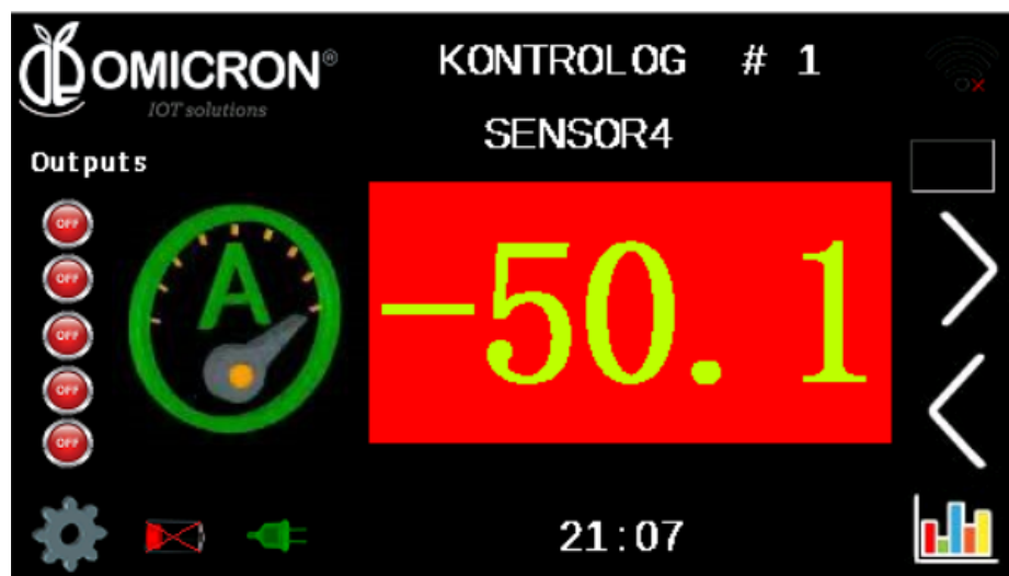
Figure 8-1 Outliers associated with sensors that are not properly connected
