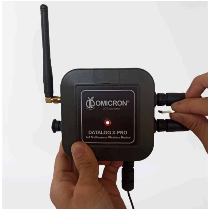
Figure 2-5 Proper position to locate the programming magnet near the Datalog X-PRO
