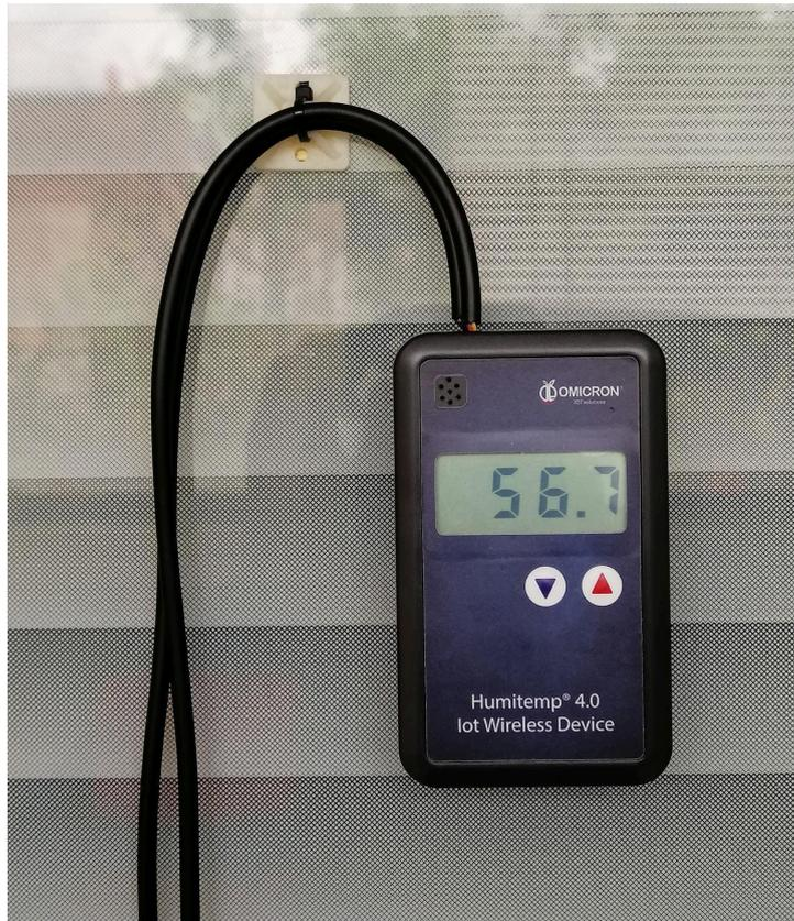
*Figure 2-7 Humitemp® wall mounting.*
