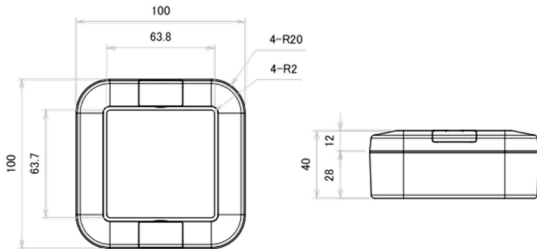
Dimensions in mm. Enclosure molded from resistant ABS material.
