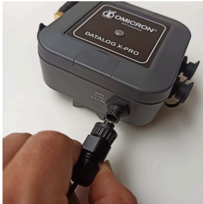
Figure 4-1 AC/DC Adapter Connection
